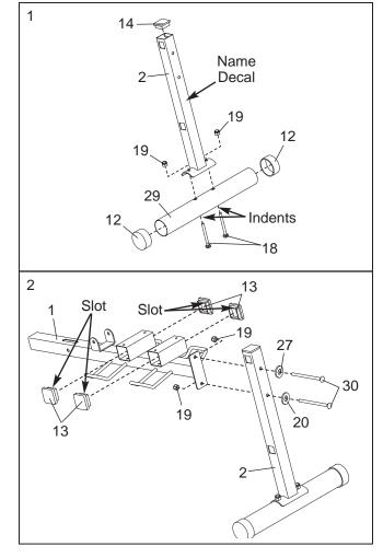
3. Press two 50mm Round Outer Caps (12) onto the ends of the Silver Stabilizer (4).
